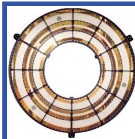
3: The High Energy Transmission Grating on the Chandra X-Ray Observatory (left) uses gold nanostructures to produce fine spectra. Developing this instrument led to a host of other detectors, and the nanoruler for making the largest high-precision gratings, such as this 91×42 cm grating made for laser pulse compression at Osaka University (above).
